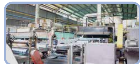
Foam Oven Expanding Machine (XLPE-Chemically CrossLinking polymer Process)
